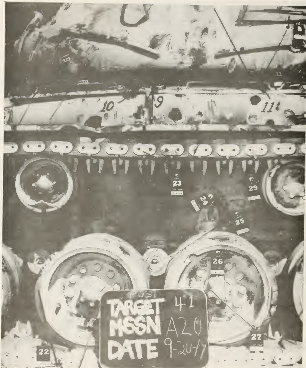
FIGURE 19. Jammed Turret caused by Impacts 9, 10, and 11, Tank 41.
